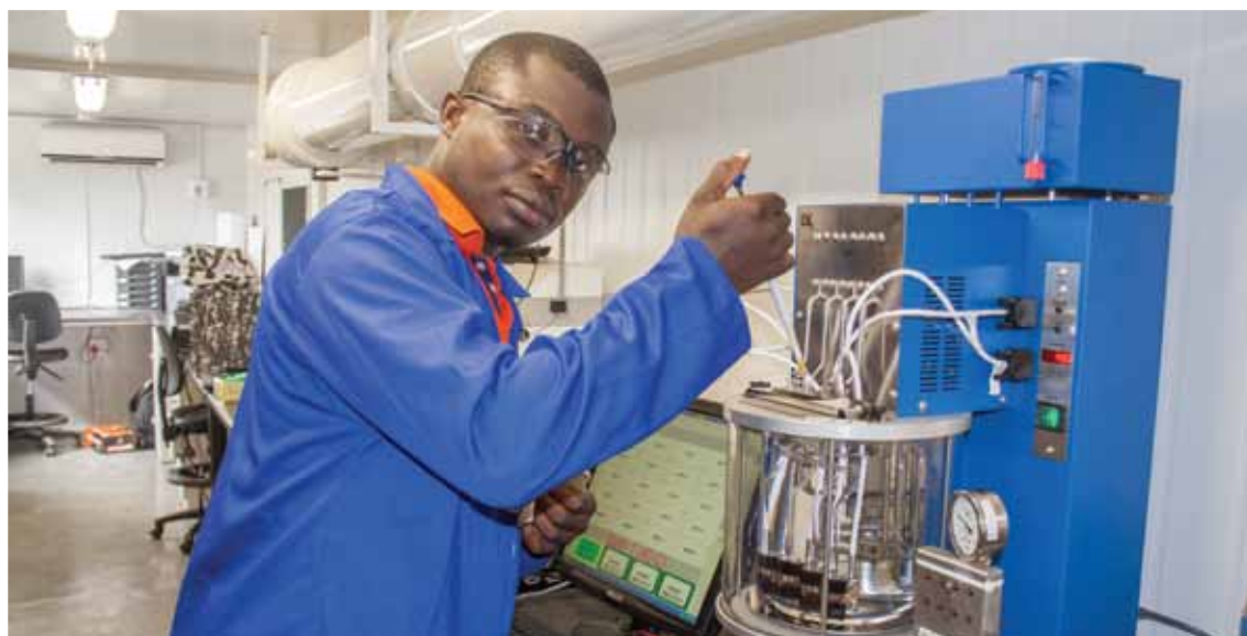
Daniel Bookye, customer sales and support officer for WearCheck Ghana, calibrates a modern software-controlled viscometer bath in WearCheck's first laboratory in West Africa, which opened recently. WearCheck Ghana offers oil analysis, an on-site sampling service and a 24-hr sample turnaround time
