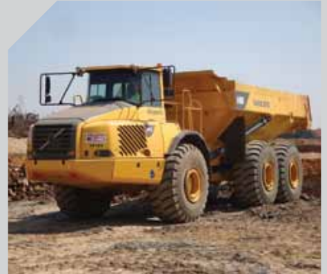
Middelburg-based mining contractor Atlantis Mining has their fleet of earth-moving vehicles on WearCheck's oil analysis programme. The engine of this Volvo A40D was recently saved through the early discovery of component wear during WearCheck's analysis of oil samples from the vehicle.
