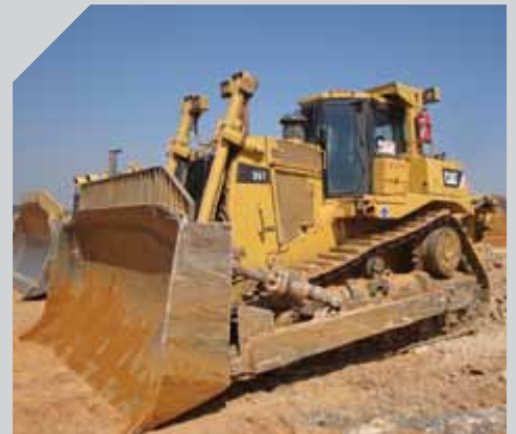
The final drives on one of Atlantis Mining's Caterpillar D9T bulldozers were recently repaired before failure thanks to timely detection of bearing wear through WearCheck's oil analysis programme.
